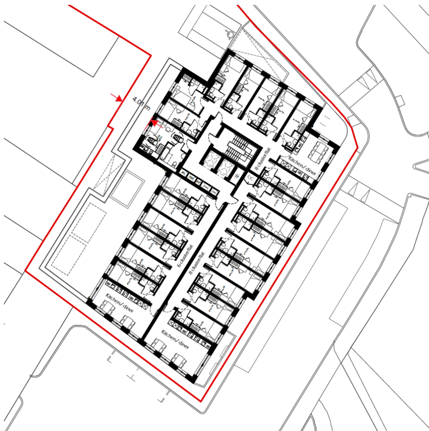
3 rd – 6 th floor plan for the appeal scheme showing the narrowest set back for a window.
